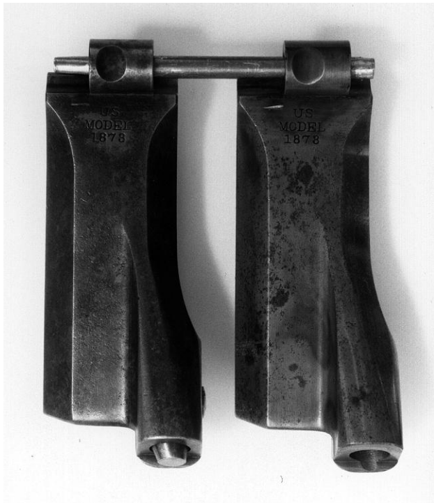
LEFT: Experimental Block. RIGHT: Service Block. Both blocks are stamped "U S /MODEL /1873." In each case, the "3" is stamped deep enough to look like an "8" which was common for blocks found on trapdoors produced in the 1882-1885 period. The top view does not indicate any apparent differences. Breech blocks from the Tom Trevor collection. Photographs by Don Harpold.
