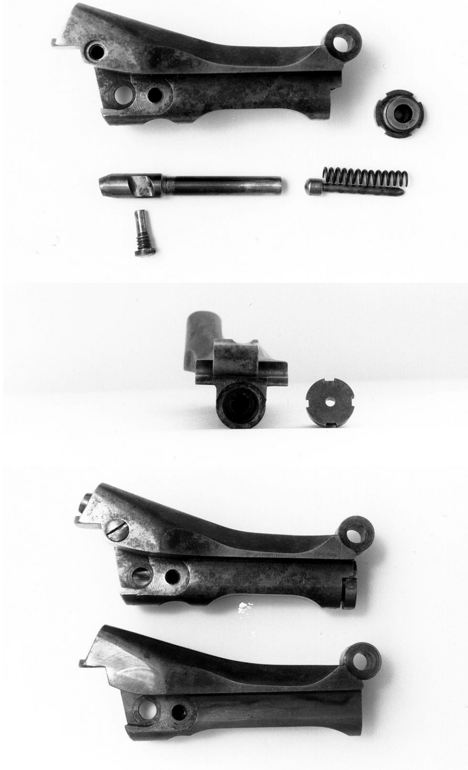
TOP: The experimental block and associated parts are clearly displayed. The firing pin tip is retained by the spring that resides against the inside of the block's detachable face plate. The upper portion of the firing pin is retained like that of the service block except the side of the screw shaft does the retaining. MIDDLE: The block recess for the spring and firing pin tip is visible. BOTTOM: The height difference in the underside arch is clearly visible and the face plate, spring and firing pin tip have been inserted into the block. Breech block is from the Tom Trevor collection. Photographs by Don Harpold.
